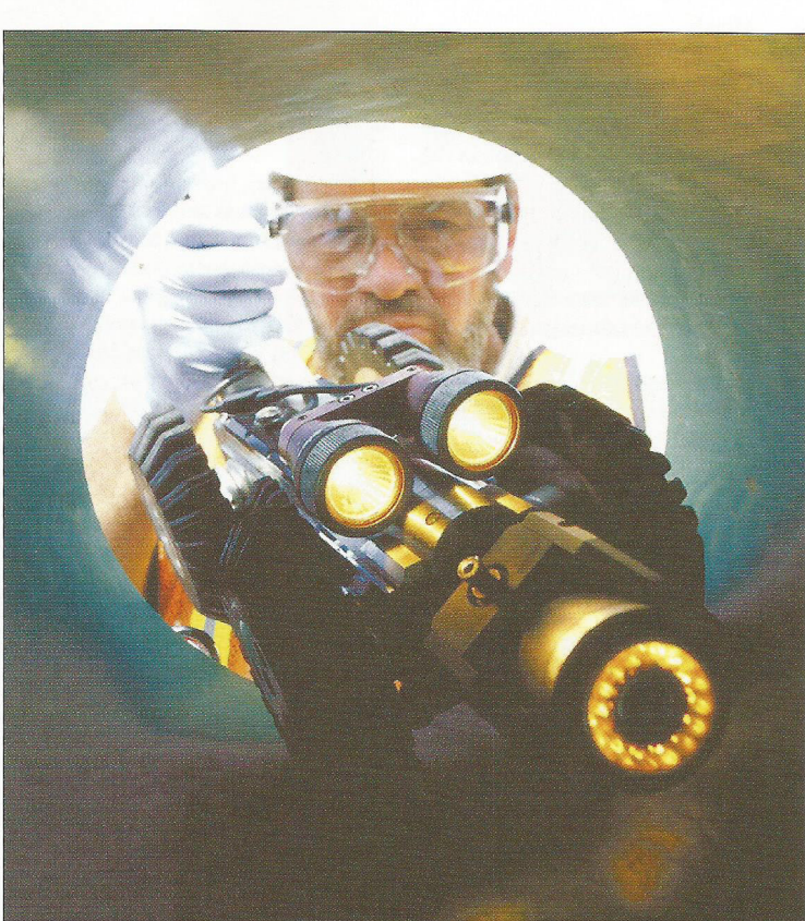
Capital City's video inspection equipment includes small, steerable Rover cameras and crawlers, 12 inches long and weighing less than 25 pounds.
